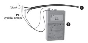
Insulation resistance measurement
