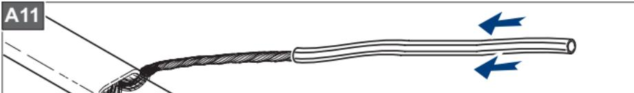
Put the green-yellow 160mm-long tube onto the twisted protection screen.
